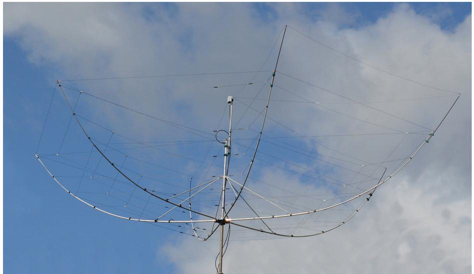
PHOTO 1: The finished Hexbeam looks a bit like an upturned umbrella.
